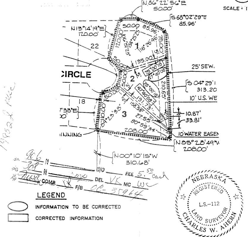
This is to certify that the angle encircled on this plat was shown in error on the original platting of Skyline Woods 2nd Addition Replat 3 and I further certify that the distance enclosed within a rectangle as shown on this plat is true, correct, and the originally intended angle.
