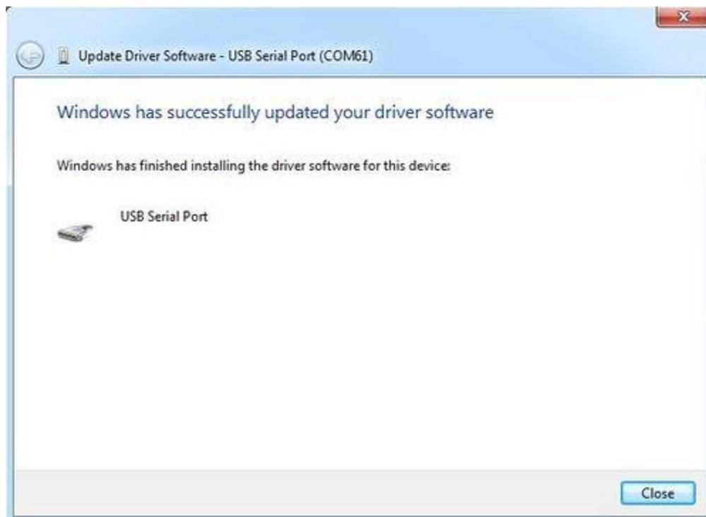
You can check that the drivers have been installed by opening the Windows Device Manager. Look for a "USB Serial Port" in the Ports section.
