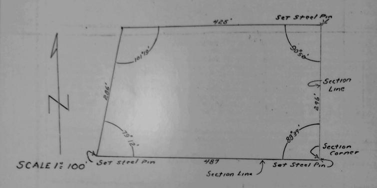
COMMENCING AT THE SECTION CORNER COMMON TO SECTIONS 29,30,31 & 32,T 7N-R18W & WEST BETWEEN SECTIONS 30 & 31 ON SECTION LINE A DISTANCE OF 487 FLET.INTERIOR ANGLE EQUALS 88 DEGREES & 39 MINUTES.(SOUTHWEST CORNER OF TRACT)
