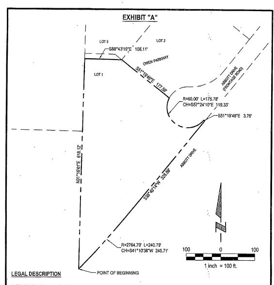
A TRACT OF LAND LOCATED IN PART OF LOT 1, OWEN PARKWAY, A SUBDIVISION LOCATED IN THE PART OF THE SW1/4 OF THE SW1/4 OF SECTION 21, AND PART OF THE NW1/4 OF THE NW1/4 OF SECTION 28, ALL LOCATED IN TOWNSHIP 75 NORTH, RANGE 44 WEST OF THE 5TH P.M., POTTAWATTAMIE COUNTY, IOWA, PARTICULARLY DESCRIBED AS FOLLOWING:
