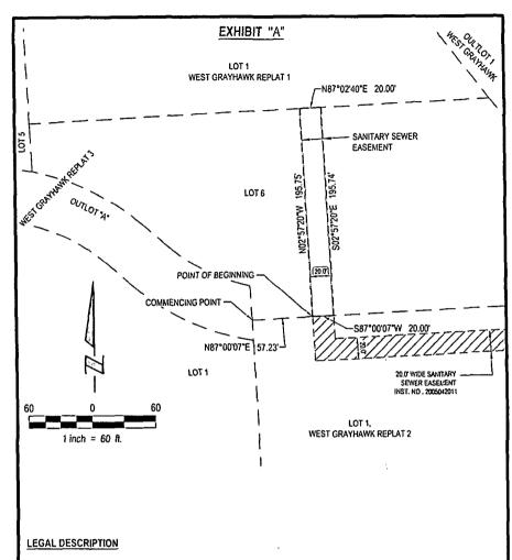
A 20.0 FOOT EXISTING SANITARY SEWER EASEMENT LOCATED IN LOT 6, WEST GRAYHAWK REPLAT 3, A SUBDIVISION LOCATED IN THE NE1/4 OF SECTION 11, TOWNSHIP 15 NORTH, RANGE 11 EAST OF THE 6TH P.M., DOUGLAS COUNTY, NEBRASKA, MORE PARTICULARLY DESCRIBED AS FOLLOWS:
