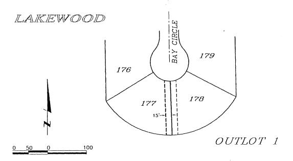
PERMANENT DRAINAGE AND STORM SEWER EASEMENT TO SID 180
