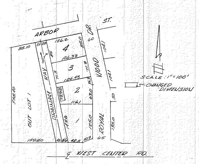
This is to certify that part of the dimensions of Lot 2, Royalwood Estates, were shown in error on the original platting and to further certify that the following plat correctly shows the originally intended lot dimensions.
