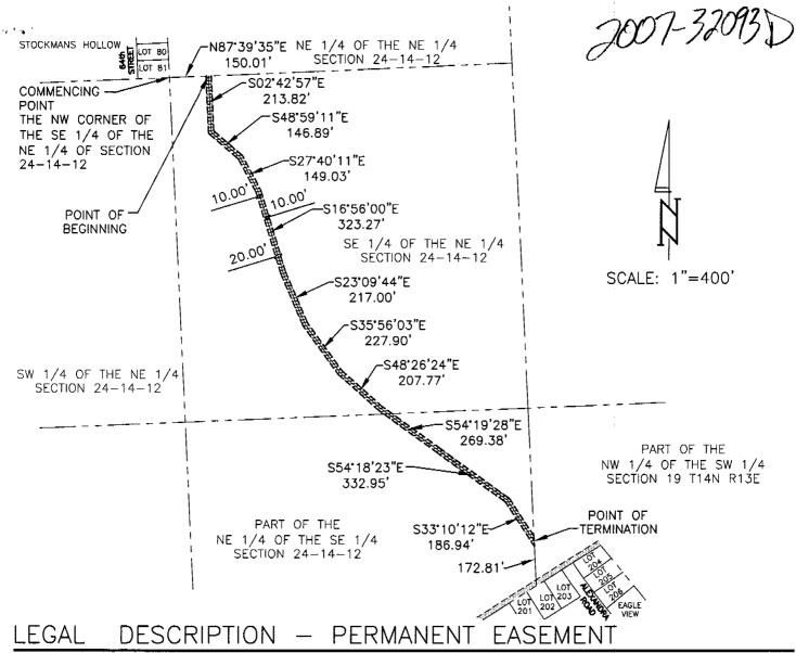
A 20.00 FOOT WIDE STRIP OF LAND LYING IN THE SE 1/4 OF THE NE 1/4 AND IN THE NE 1/4 OF THE SE 1/4, ALL IN SECTION 24, T14N, R12E OF THE 6th P.M., SARPY COUNTY, NEBRASKA, THE CENTERLINE OF SAID 20.00 FOOT WIDE STRIP OF LAND BEING DESCRIBED AS FOLLOWS:
