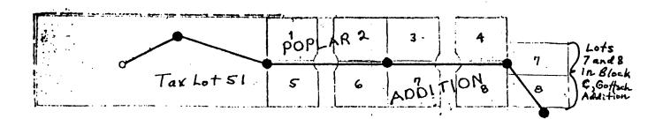
Note - The darkened line above and circled portions connected thereto denote the sewer or drain lines or pipes as well as the manhole cleanout servicing same which are collectively referred to as "sewer lines" in said DEDICATION AND EASEMENT.
