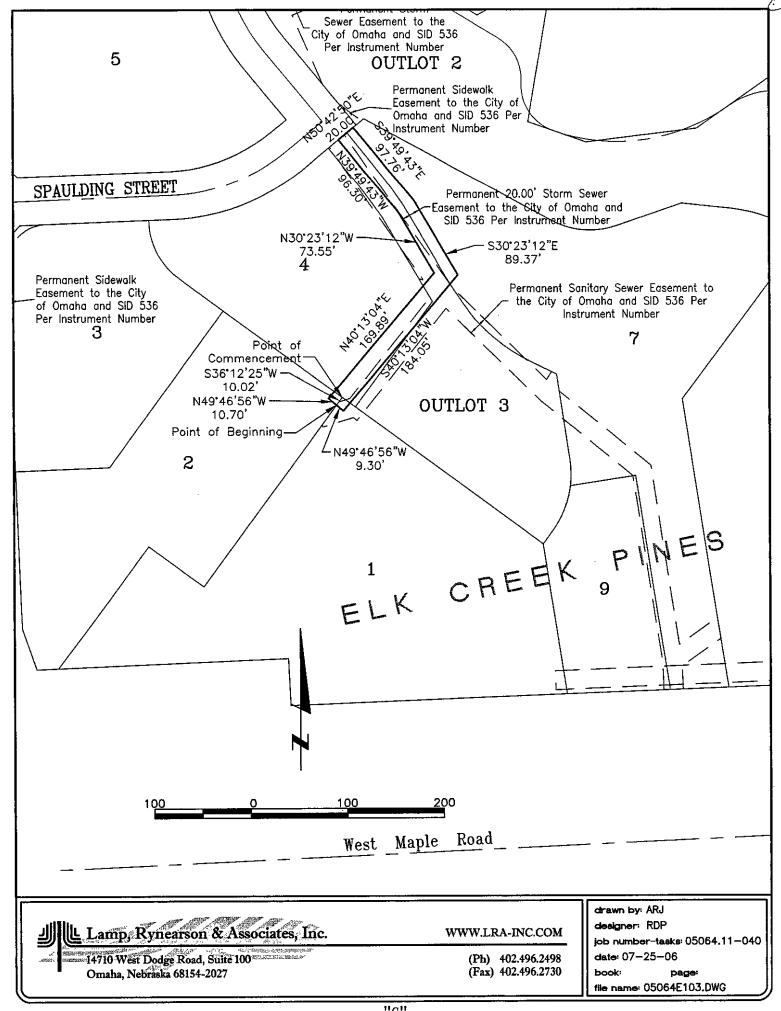
A permanent easement twenty foot in width for the construction and maintenance of storm sewers over that part of Lots 7 and 8 AND Outlot 2, ELK CREEK PINES, a subdivision, as surveyed, platted and recorded in Douglas County, Nebraska, the perimeter of which is described as follows:
