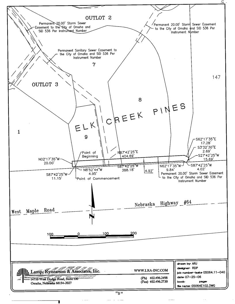
A permanent easement twenty foot in width for the construction and maintenance of storm sewers over that part of Lots 1, 2, 4, and 7 AND Outlot 3, ELK CREEK PINES, a subdivision, as surveyed, platted and recorded in Douglas County, Nebraska, the perimeter of which is described as follows:
