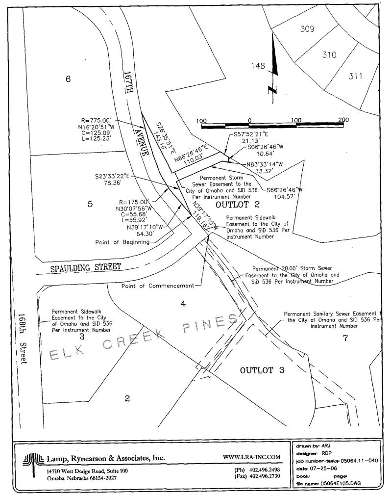
A permanent easement twenty foot in width for the construction and maintenance of storm sewers over that part of Outlot 2, ELK CREEK PINES, a subdivision, as surveyed, platted and recorded in Douglas County, Nebraska, the perimeter of which is described as follows:
