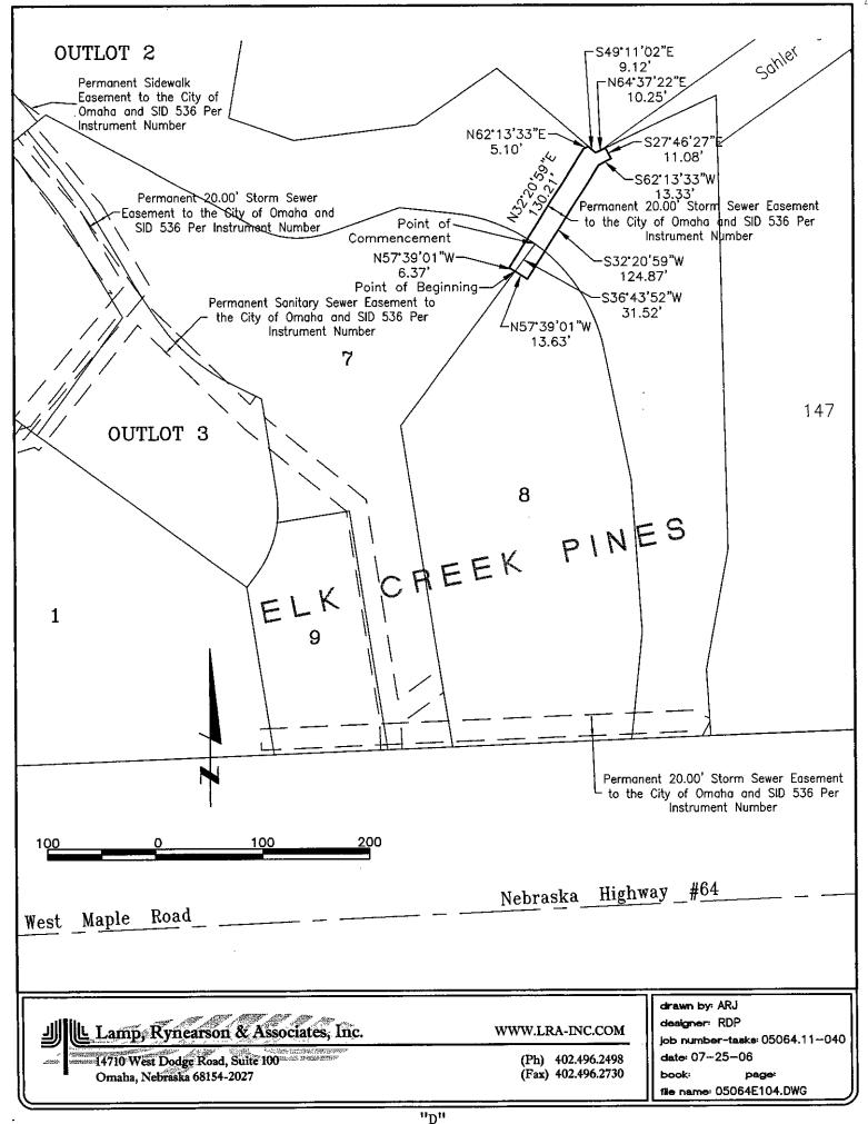
A permanent easement for the construction and maintenance of storm sewers over that part of Outlot 2, ELK CREEK PINES, a subdivision, as surveyed, platted and recorded in Douglas County, Nebraska, described as follows:
