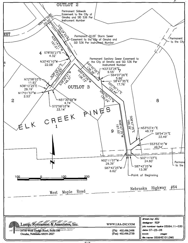
A permanent easement twenty foot in width for the construction and maintenance of storm sewers over that part of Lots 1, 7, 8, and 9 AND Outlot 2, ELK CREEK PINES, a subdivision, as surveyed, platted and recorded in Douglas County, Nebraska, the perimeter of which is described as follows:
