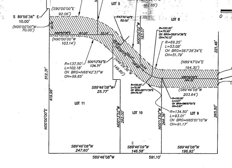
A STRIP OF LAND FOR PERMANENT RECIPROCAL ACCESS EASEMENT, UTILITY EASEMENT AND STORM SEE EASEMENT PURPOSE; BEING PART OF LOTS 1 THROUGH 11, WEST POINT REPLAT 1, A PLATTED AND REING THE SW1/4 OF SECTION 2, T15N, R11E OF THE 6TH P.M., DOUGLAS COUNTY, NEBRASKA, BEING MOIDESCRIBED AS FOLLOWS:
