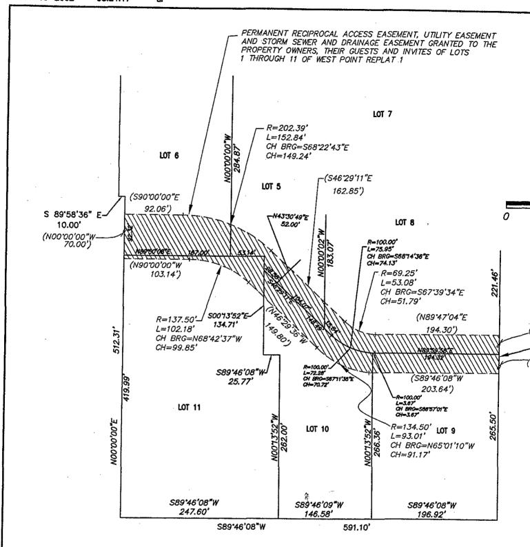
A STRIP OF LAND FOR PERMANENT RECIPROCAL ACCESS EASEMENT, UTILITY EASEMENT AND STORM SE EASEMENT PURPOSE; BEING PART OF LOTS 1 THROUGH 11, WEST POINT REPLAT 1, A PLATTED AND RE IN THE SW1/4 OF SECTION 2, T15N, R11E OF THE 6TH P.M., DOUGLAS COUNTY, NEBRASKA, BEING MODESCRIBED AS FOLLOWS:
