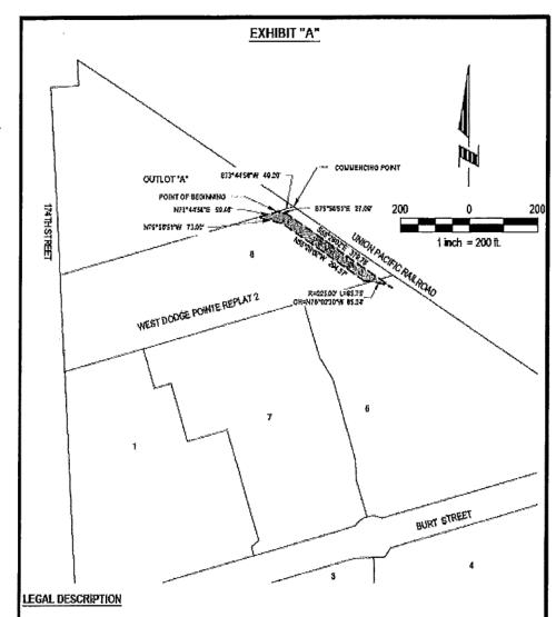
A STORM SEWER EASEMENT SEING LOCATED IN PARTS OF LOT 6 AND 8, WEST DODGE POINTE REPLAT 2, A SUBDIVISION LOCATED IN PART OF THE SELVA OF THE SELVA, PART OF THE SWIM OF THE SELVA AND PART OF THE NIM WA OF THE SELVA, LOCATED IN SECTION 16, TOMOSHIP 15 NORTH, RANGE 11 EAST OF THE 6TH P.M., DOUGLAS COUNTY, NEBRASKA. MORE PARTICULARLY DESCRIBED AS FOLLOWS:
