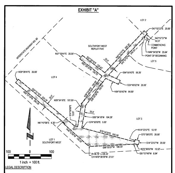
A 20.0 FOOT STORM SEWER AND DRAINAGE EASEMENT LOCATED IN LOTS 2 THROUGH 5, SOUTHPORT WEST REPLAT FIVE, A SUBDIVISION LOCATED IN THE SW1/4 OF SECTION 18, TOWNSHIP 14 NORTH, RANGE 12 EAST OF THE 6TH P.M., SARPY COUNTY, NEBRASKA. MORE PARTICULARLY AS DESCRIBED AS FOLLOWS:
